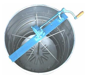
It is not necessary to fill the extractor with 10 frames each time, as is works equally well (and is lighter to turn) with a smaller number, as long as the load is balanced. Being hand turned, it is not limited to a place with electricity. It can travel out to the bees with you.
